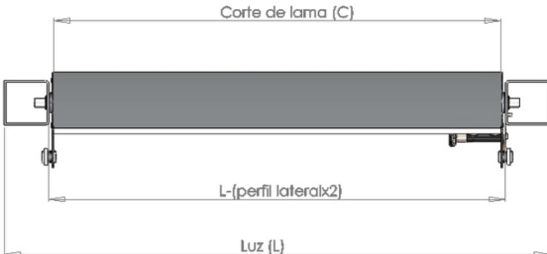
$C = L - (\text{perfil lateral} \times 2) - 10\text{mm}$
