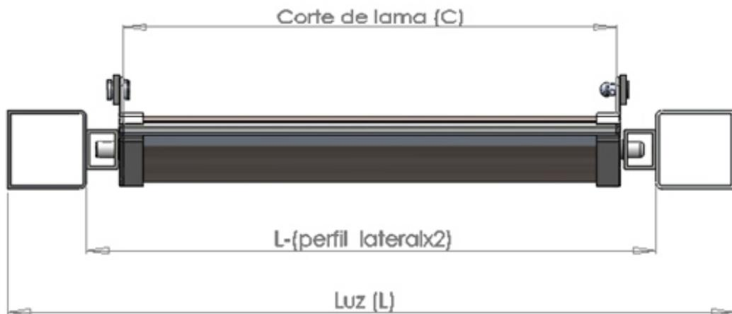
$C = L - (\text{perfil lateral} \times 2) - 40\text{mm}$
